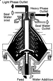
fining centrifuges, it is hermetic which avoids oxidation during processing and subsequent degradation problems.
